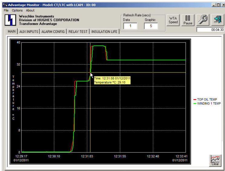
Plate 106. The hover dialog works on the larger graphic, but here are times when signals overlap and it can be hard to pick out an individual signal. There is a plot expansion tool for this situation.
