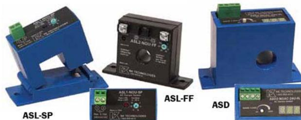
New NK Technologies AC current switches allow simplified setup on a de-energized circuit. Sense from 1A to 150A, in both solid-core and split-core styles, with the **ASL** series. A single-turn pot provides the trip current adjustment. The trip setting is indicated on the label and always visible. ASL models are self-powered from the monitor circuit. Choose a normally open or normally closed solid-state output (AC/DC) when ordering.
