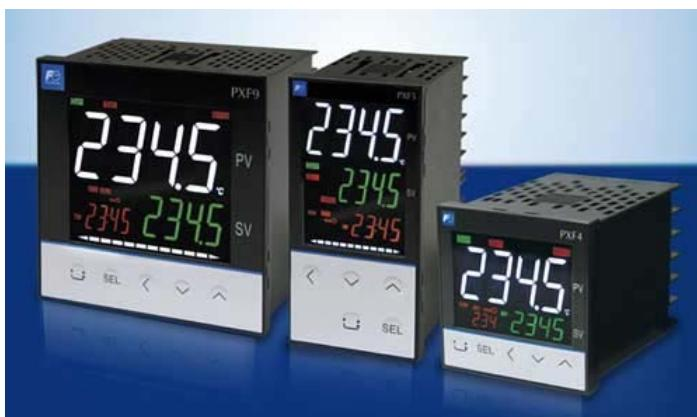
The new **Fuji** PXF Process Controllers are fast, compact & user friendly. Three models feature a large, bright color display, universal input and 50ms sampling rate. Other features include 7 control methods, 64 ramp/soak segments, 2 control outputs and up to 4 alarm outputs. Options include RS485 Modbus communications, digital inputs and motorized valve control versions. Initial setup can be done via USB without external power.
