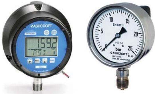
Ashcroft offers pressure transmitters with either digital or analog readout. The **Ashcroft 2074** family is available in 3" and 4.5" sizes, with 1/4% FS accuracy. Both sizes have a large 5 digit display with selectable engineering units. Choose battery, loop or DC power when ordering. The **Ashcroft T5500E** has a 4" dial and Grade 2A (1/2% FS) accuracy. The transmitter section is externally powered from 12-30VDC.
