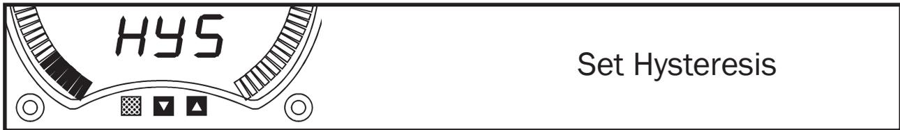
Hysteresis may be set in 0.1% increments from 0 to 10% of Full Scale. Attempting to increment past 10% will enable latching for all alarms (infinite hysteresis).
