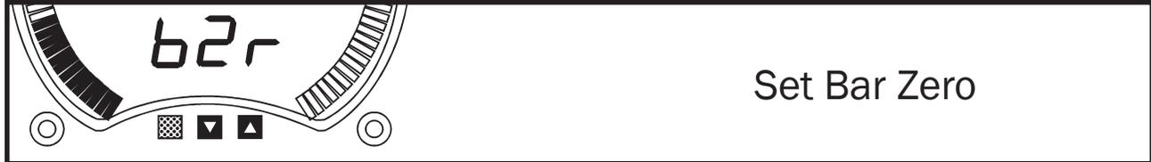
The BarGraph zero display point may be set to a percentage of Full Scale. This is not a calibration function. It only affects the value the BarGraph will display at the lowest end of the bar display. This setting can be used to limit the lowest value that the BarGraph will display. This function will not be enabled or displayed unless barform has been set to Deviation or Variable barform (see barform function).
