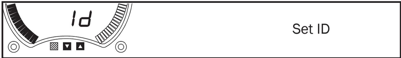
This function is used to set BarGraph communication ID. Each BarGraph hooked to the communication lines must have its own unique ID to distinguish it from other units.
