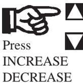
If latching was enabled for this setpoint in Supervisor Setup and the alarm is latched (**L L H**), pressing either the INCREASE or DECREASE key will release the alarm. Pressing ENTER/SAVE without pressing INCREASE or DECREASE will leave the alarm in a latched state and display the setpoint value.
