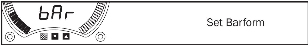
This function allows the user to set the display format. The most common display format is bottom zero, ie; starts at the bottom (or most left for circular or horizontal displays) and increasing up (towards the right for circular or horizontal displays). The BarGraph zero point can be located or referenced anywhere on or off the scale in this setup.
