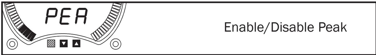
Peak/Valley allows the BarGraph to display the highest (Peak) and lowest (Valley) level during the reading cycle, as determined by the reset.
