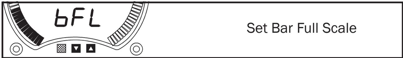
The BarGraph Full Scale display point may be set to a percentage of Full Scale for measurement. This is not a calibration command. It only affects the BarGraph display. This command and the Set Bar Zero function may be used to limit the values shown on the bar display to a specific region of interest. This function will not be enabled or displayed unless barform has been set to Deviation or Variable barform (see Set Barform function).
