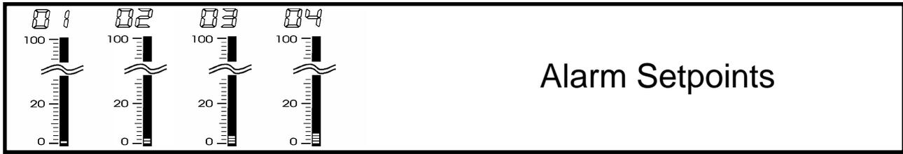
Up to four alarm setpoints are provided, depending on the exact model of BarGraph™ ordered and the options supplied. Each of the available setpoints may be programmed for a specific value under Supervisor Setup.
