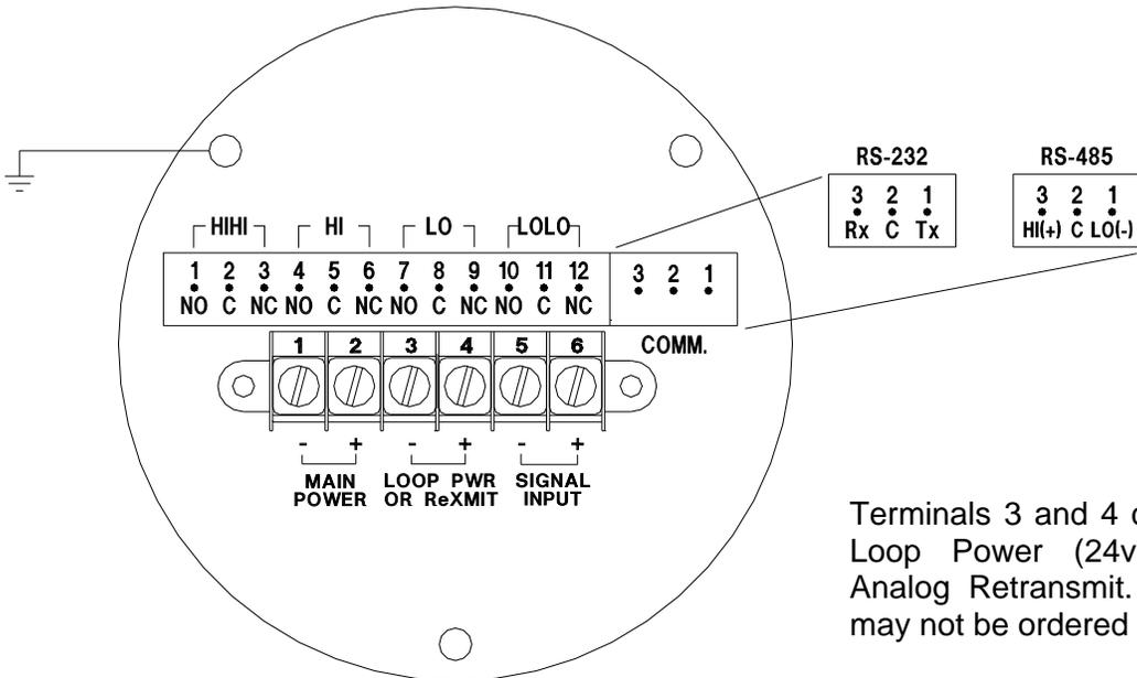
Terminals 3 and 4 can be used for Loop Power (24vdc supply) or Analog Retransmit. These options may not be ordered together.
