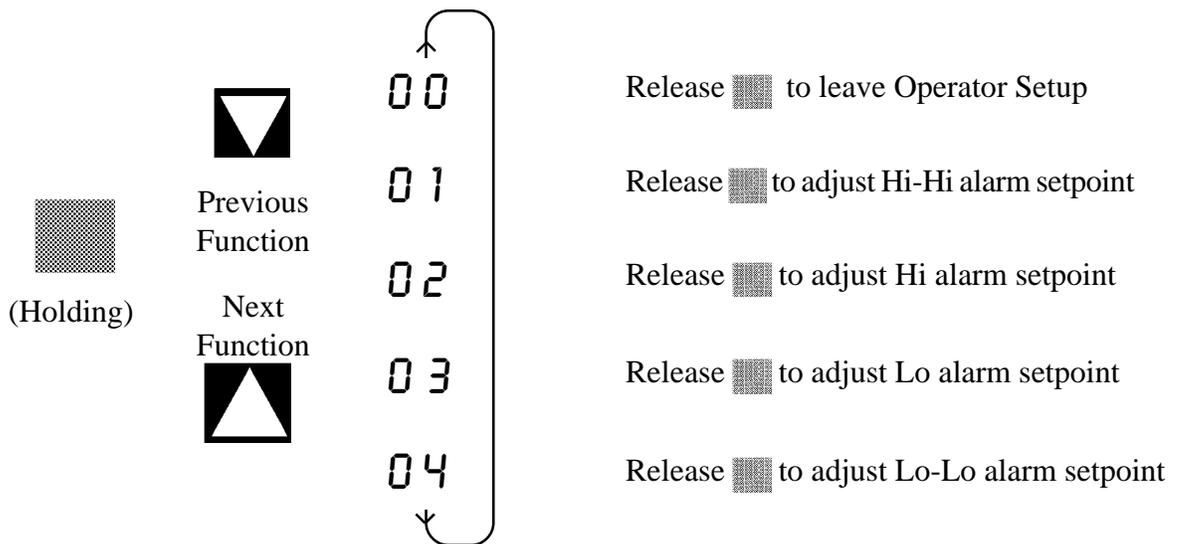
Releasing the ENTER key while any of the above are displayed will display the current setting and allow it to be modified. Setting each of the above functions is described on the following pages.
