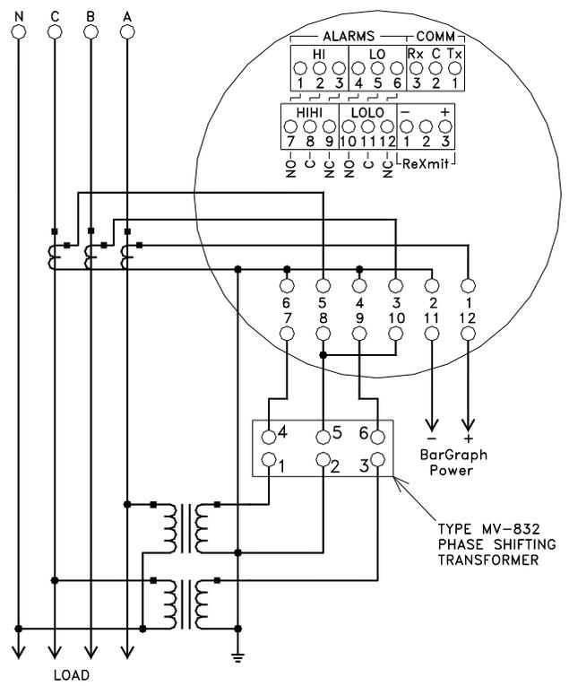
3 Phase 4 Wire with Phase Shifting Transformer
