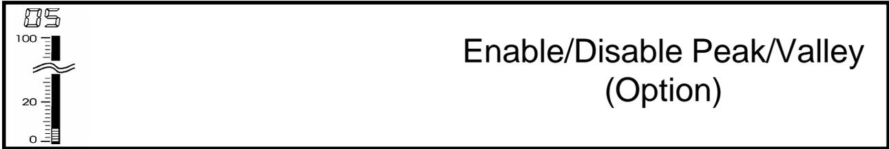
Peak/Valley allows the BarGraph™ to display the highest (Peak) and lowest (Valley) level during the reading cycle, as determined by the reset. This function will only be available if the BarGraph™ was ordered with Peak/Valley option.
