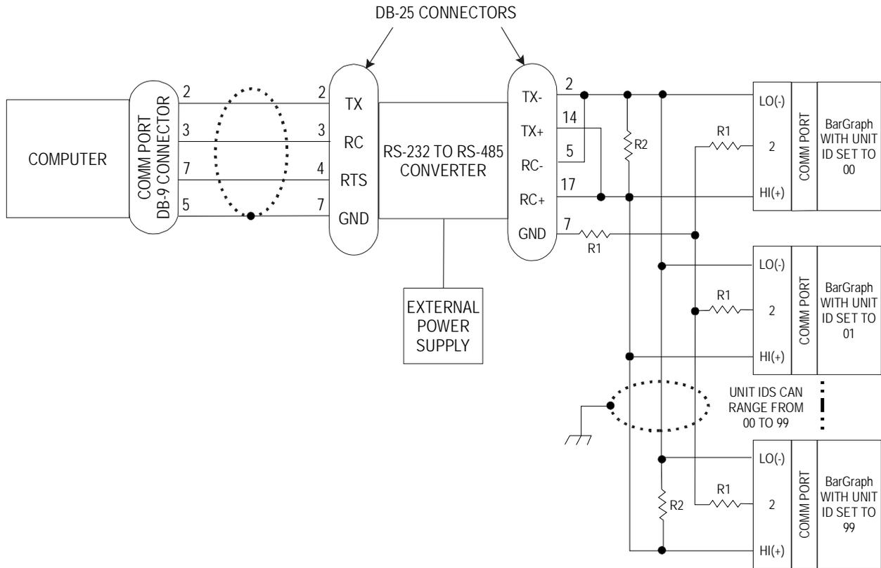
1. Add 120 ohm termination resistors (R2) at the output of the converter and to the terminals of the last BarGraph on the branch circuit.
