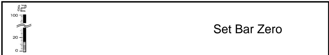
The BarGraph™ zero display point may be set to a percentage of Full Scale. This is not a calibration function. It only affects the value the BarGraph™ will display at the lowest end of the bar display. This setting can be used to limit the lowest value that the BarGraph™ will display. This function will not be enabled or displayed unless barform has been set to Deviation or Variable barform (see barform function).
