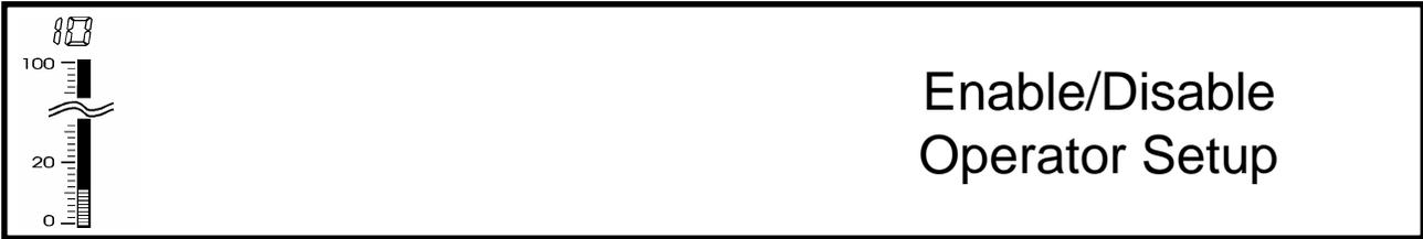
Operator Setup can be enabled or disabled through this function. If Operator Setup is disabled, setpoints for alarms 1 through 4 can no longer be set without jumper JA1.
