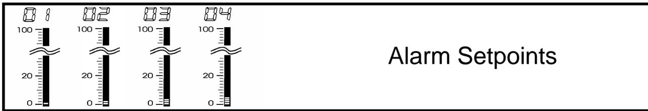
Up to four alarm setpoints are provided, depending on the exact model of BarGraph™ ordered and the options supplied. Each of the available setpoints may be programmed for a specific value under Operator Setup if enabled (see Enable/Disable Operator Setup in Section 4.2).
