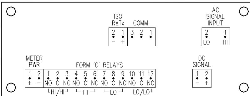
AC or DC Volt, Millivolt, Amp, Milliamp or Line Frequency Signal Inputs (OP6)
