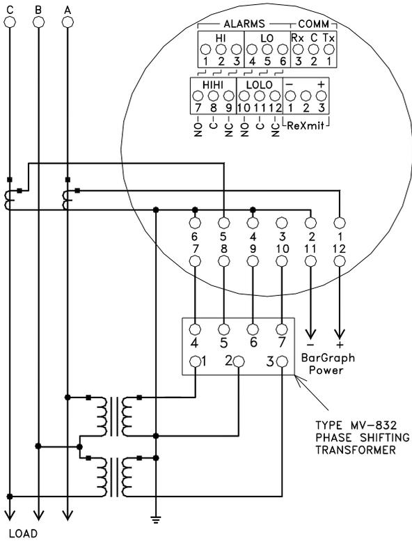
3 Phase 3 Wire with Phase Shifting Transformer
