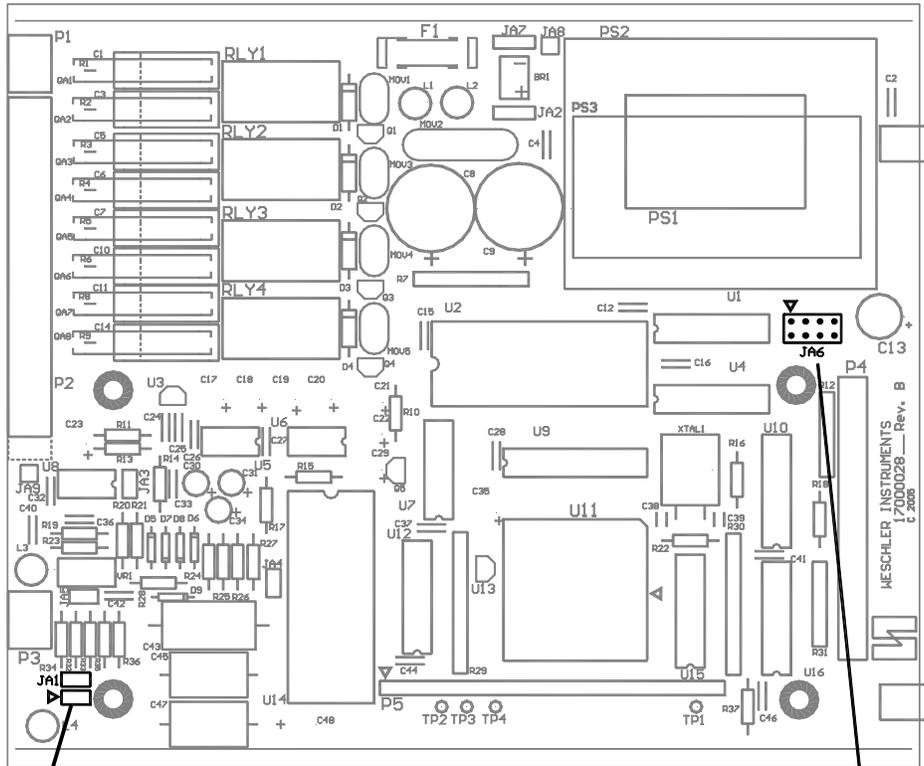
JA-1: Install a Jumper to Enter Supervisory Set-up
