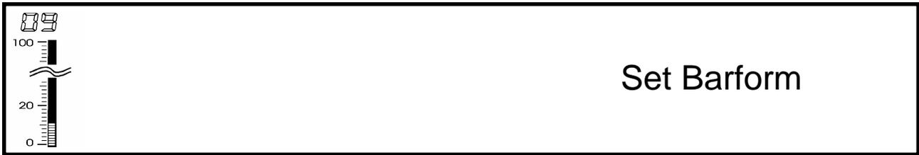
This function allows the user to set the display format. The most common display format is bottom zero, ie; starts at the bottom (or left) and increasing up (or to the right). The BarGraph™ zero point can be located or referenced anywhere on or off the scale in this setup.
