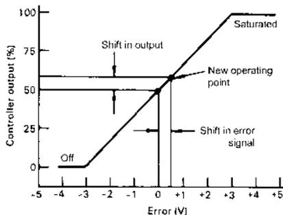
Controllers with reset (integral) action will automatically recenter the proportional band around the offset bias level. An integral mode controller responds to the integral of the difference between the setpoint and measured value. The adjustable parameter for integral control is the integral time  $T$ , or the reset rate  $1/T$ . The integral mode is sometimes used as a single mode of control but is more
