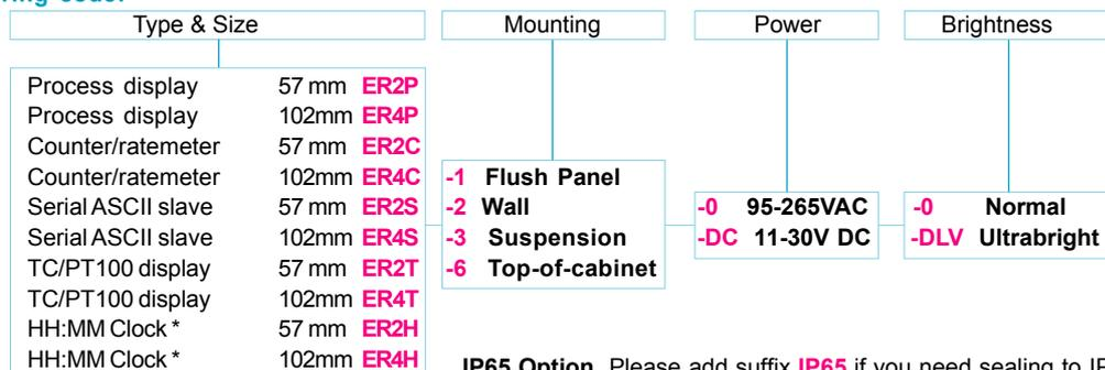
For example model **ER4P-2-DC-0** is a wall mount 102mm process display, DC power, normal brightness.
