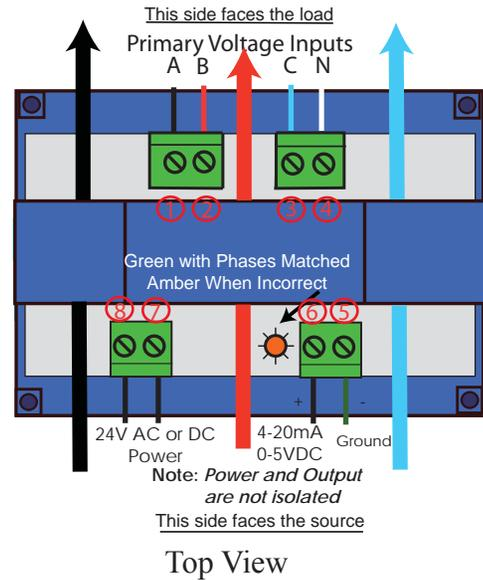
The APT-TH power transducer provides current sensing windows with an inside diameter of 0.74 inches. This should be large enough to accommodate a single conductor carrying 200 amps.
