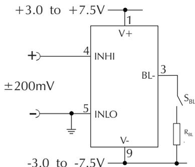
Measuring a single ended input voltage referenced to a split supply, i.e. the input voltage and the meter's power supply share the same 0V rail. Ensure solder link LCOM is open.
