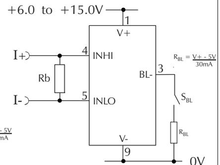
Measuring a current from a circuit which is floating with respect to the DPM's supply, i.e. the current and the meter's power supply are isolated from each other. Ensure solder link LCOM is closed.
