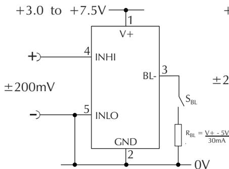
Measuring a single ended input voltage referenced to supply, i.e. the input voltage and the meter's power supply share the same 0V rail. Ensure solder link LCOM is open.
