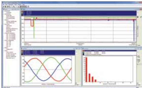
Real-time view of trend, waveform and status screens.
