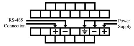
The far end can be connected to any communications device that is acting as the master, such as a computer. The unit can also be connected in parallel with other units. If you wish to use a personal computer to communicate with the *Power Series*<sup>Plus</sup> an RS-232/RS-485 converter will be needed.
