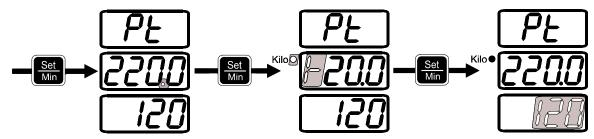
Pressing **Set** will now move you to the Confirm mode. All values will blink. If the values are correct press **Set** one last time to save them and move on to the Current Transformer settings. Pressing **Mode** at this time or at any other step in the process will restore the old PT settings.
