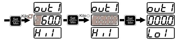
Pressing **Set** will now move you to the HI Confirm mode. The whole value will blink. If the value is correct press **Set** one last time to move on to the LO setting. Pressing **Mode** at this time or at any other step in the process will restore the old HI setting.
