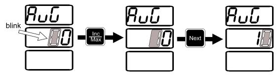
To increment the value of the digit, press Inc. Once a digit has reached 9 (nine), it will then go to 0 (zero). To move to the second digit press Next. To return to the first digit press Next again. When you have set the desired value, press Set. Both digits will blink, showing you are now in Confirm mode. If the value is correct press Set one more time to save the value and move on to the Address setting. Pressing Mode at any time before this will restore the old setting.
