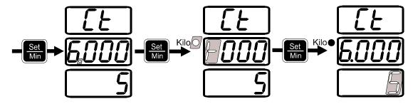
If you have a 1 Amp unit, or you have set the secondary on a 5 Amp unit, pressing **Set** will now move you to the Confirm mode. All values will blink. If the values are correct press **Set** one last time to save them and move on to the Analog Output settings. Pressing **Mode** at this time or at any other step in the process will restore the old CT settings.
