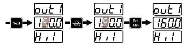
When you have set the digits as you want them, press **Set**. The decimal point will now be blinking. You can then move the decimal point to the right by pressing **Inc**. Once it has reached the last position it will jump to the first position on the next press of **Inc**.
