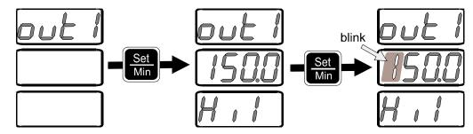
To move to the next digit press **Next**. **Next** will move you through all four digits and back to the first one, if necessary. You can increment the value of the blinking digit by pressing **Inc**. Once a digit has reached 9 (nine) it will go to 0 (zero) on the next press of **Inc**.
