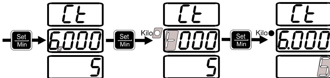
If you have a 1 Amp unit, or you have set the secondary on a 5 Amp unit, pressing **Set** will now move you to the Confirm mode. All values will blink. If the values are correct press **Set** one last time to save them and move on to the Analog Output settings. Pressing **Mode** at this time or at any other step in the process will restore the old CT settings.
