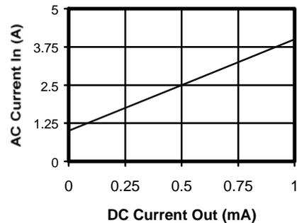
Next the CT ratio is changed to 2 to 1 (2:1). **Note** that the HI and LO automatically change to match the new ratio whenever the CT ratio is changed. So now the settings are
