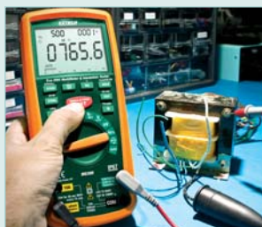
Measure the insulation resistance of transformer windings
