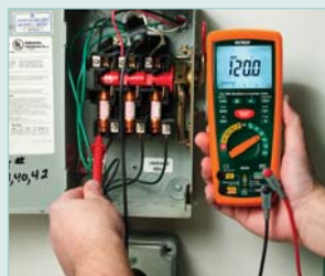
Only a True RMS meter can give accurate readings of distorted waveforms
