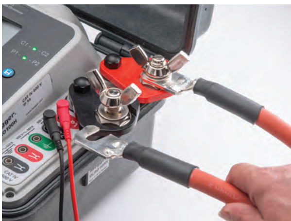
A new terminal adapter has been designed to enable the use of users own test leads.
