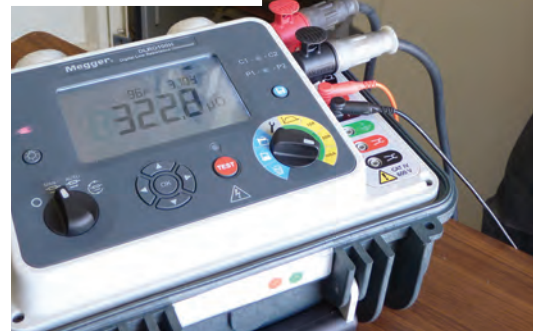
DLRO100H testing rack-mounted, 3-phase circuit breakers
