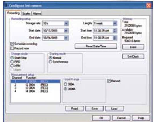
Quick and simple configuration of all functions and settings from one dialog box.
