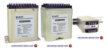
Texmate Transducers convert AC voltage, AC current and frequency signals to a DC value for easy readout or input to a SCADA system. Use these transducers with direct signals up to 5A or 600V. For higher signal levels, connect using a current transformer (CT) or potential transformer (PT). Both average and TRMS sensing models are available. TRMS sensing is recommended for input signals with distortion.
