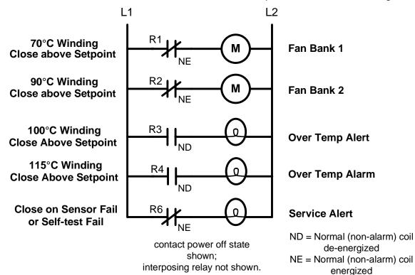
To implement, wire as shown above. Configure 2 relays for cooling fans and 3 relays for external alarms. Define the normal (non-alarmed) coil state for standard or fail-safe mode. Then set up the internal alarms for setpoint, hysteresis & delay. Link each alarm to a relay. Enable sensor failure response & effect for the alarms tied to fan stages.
