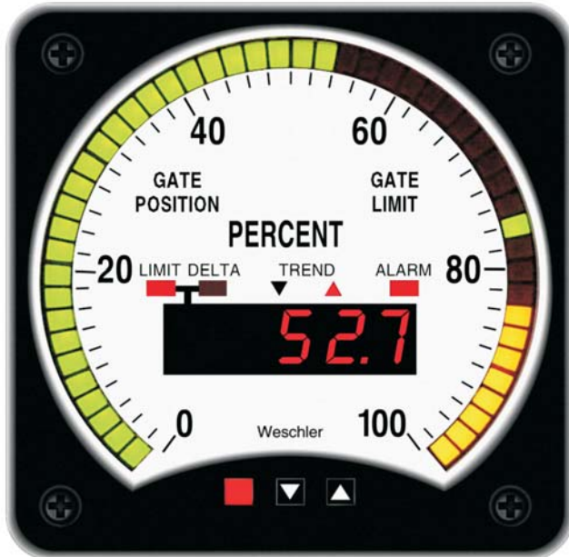
BG241 GPI with optional Trend & Alarm functions. Green bar indicates gate position. Yellow bar indicates gate limit. Single illuminated segment shows the adjustable alarm level.
