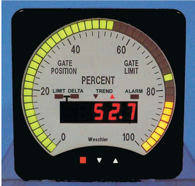
BG241 GPI with optional Trend & Alarm functions. Green bar indicates gate position. Yellow bar indicates gate limit. Single illuminated segment shows the adjustable alarm level.
