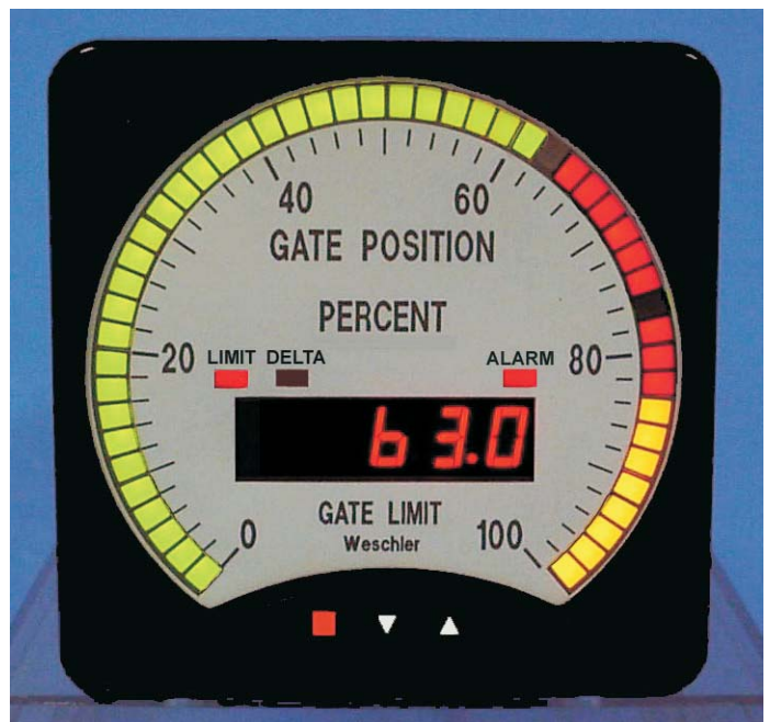
Bar changes color when gate position exceeds limit. UP button toggles digital display between position, limit & delta. Example of a custom dial shown here.
