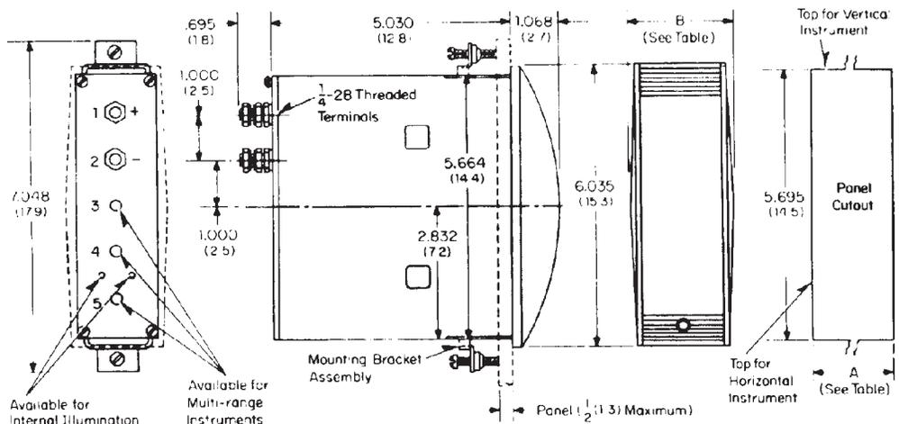
**Figure 2: Outline and Drilling Dimensions, In Inches (Millimeters)**
